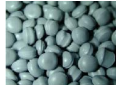
EBS1: Hartpellets Heizwert 14 -18 MJ/kg EBS 2: weichere Pellets EBS 3: Fluff
